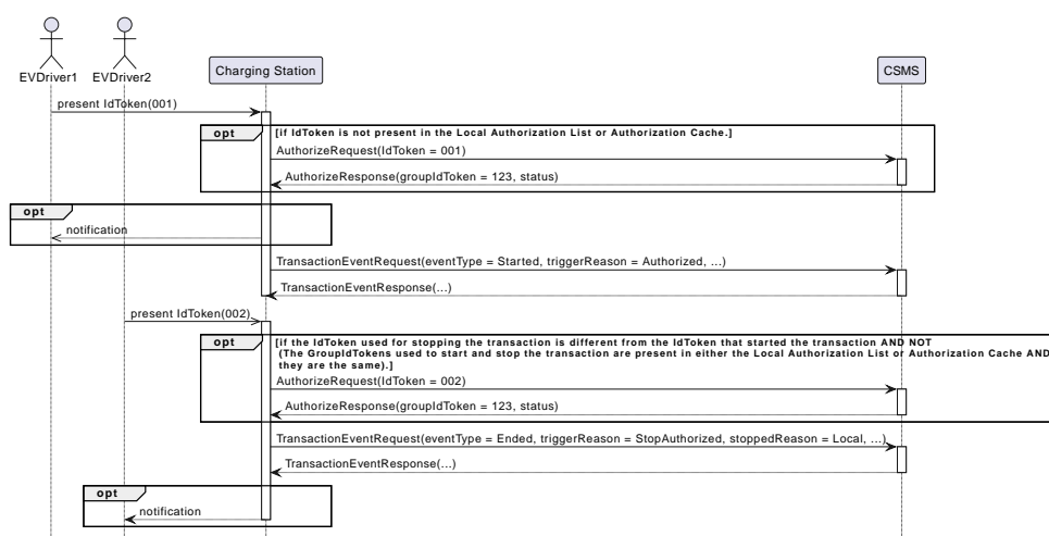
Figure 30. Sequence Diagram: Authorization by GroupId
