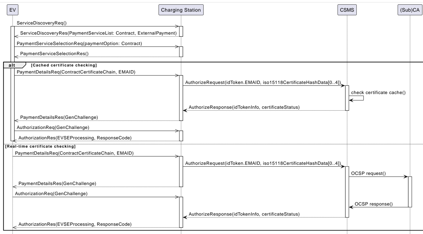
Figure 26. Authorization using Contract Certificates with ISO 15118-2
