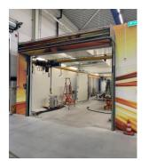
Optionally EVSE in climate chamber at - 20°C (-30°C) to + 60°C
