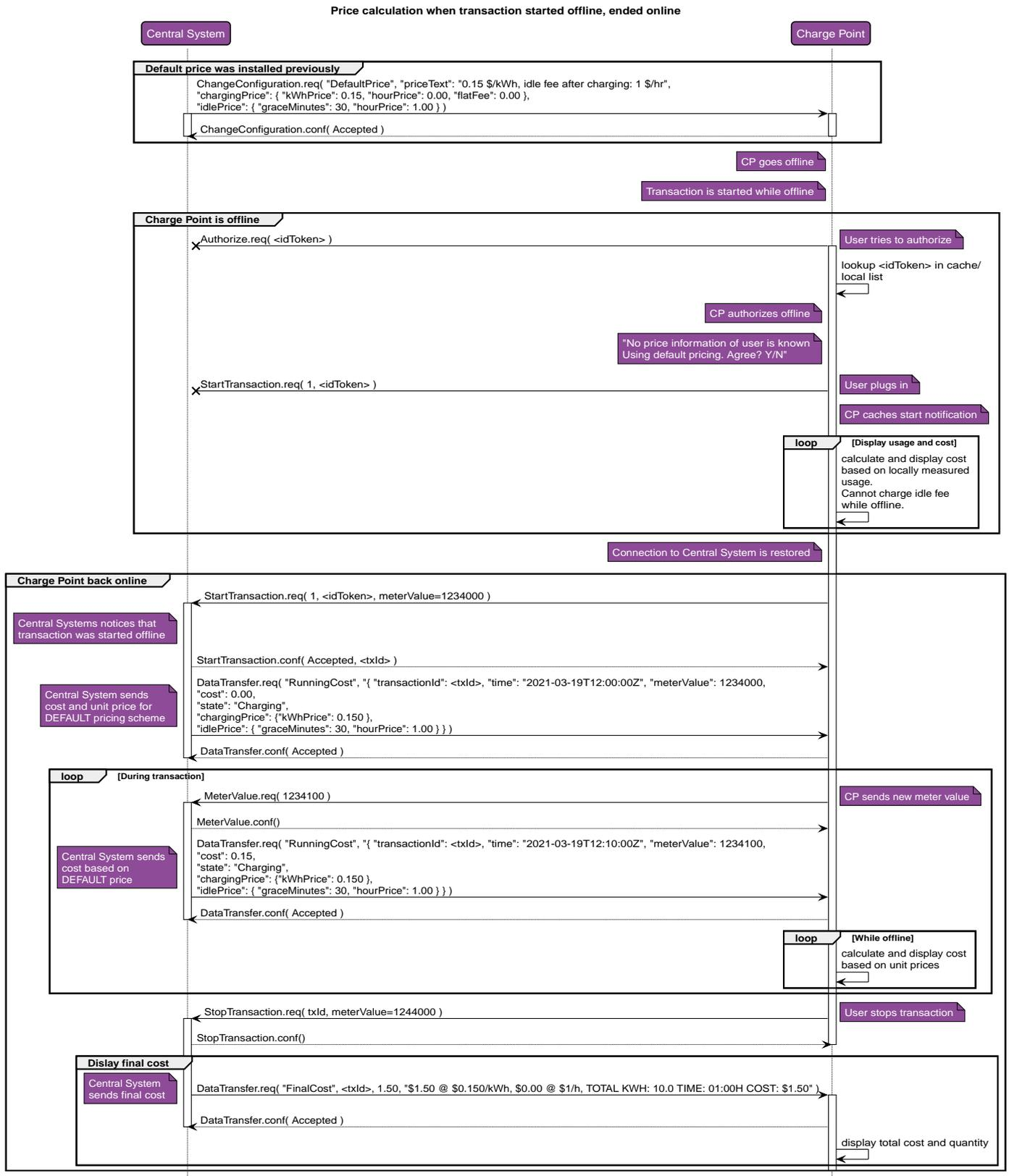
Figure 6. Price calculation for offline started transaction
