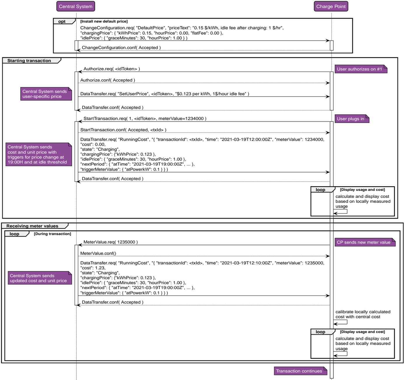
Figure 1. Price calculation during transaction
